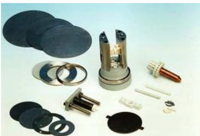
Sample holder of high temperature measuring system in van der Pauw geometry (partially assembled)
