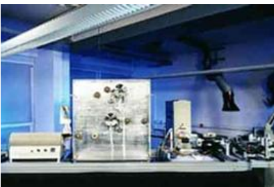
Winding machines for fabrication of ceramic matrix composites
